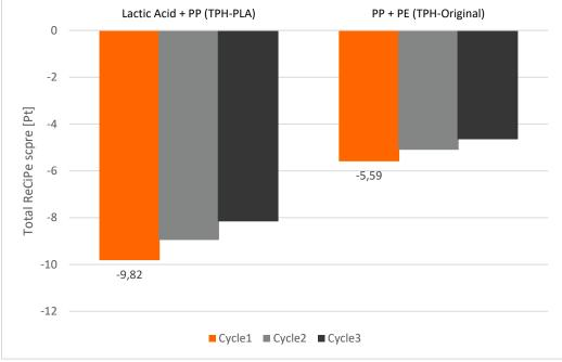
Figure 4 Comparison of PLA and original scenario - Avoided impact plastics per cycle
